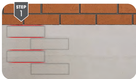
Make lines using a spirit level for the coursing of the slips.
