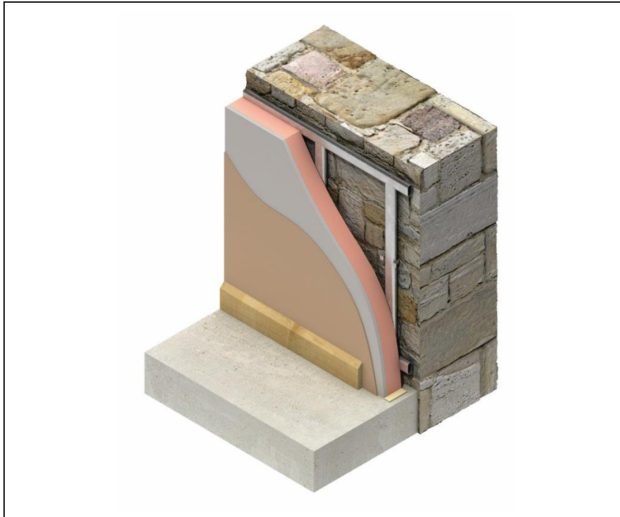
Figure 4 Wetherby internal wall insulation board fixed to metal wall liner
